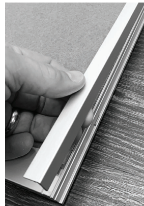
Once the cords are removed, the aluminum edge profiles can be lifted from the assembly.
